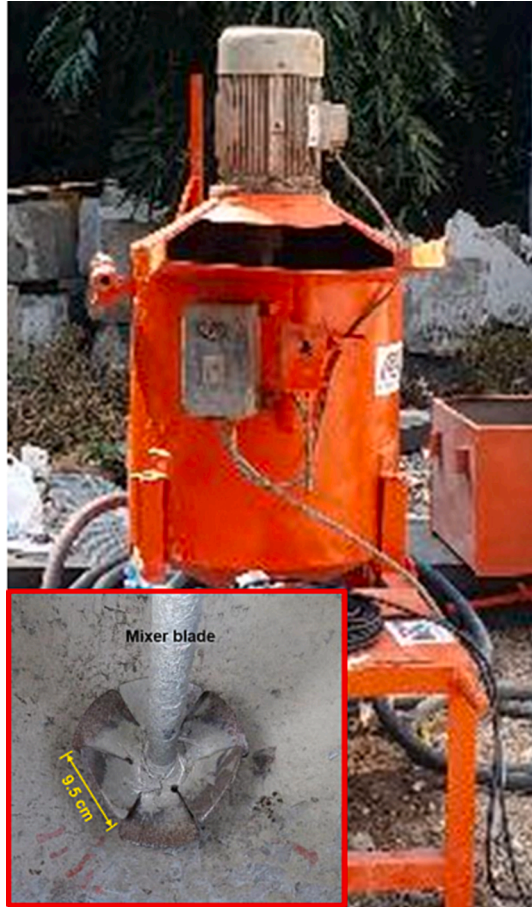
Fig. 10. Grout mixer and the blade configuration used for prototype-scale grouting studies.
